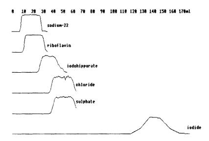
Elution profiles of 20ml aliquots containing various labelled substances. [<sup>99m</sup>Tc]pertechnetate not shown as it elutes at 450ml. Vertical scales are optical density (riboflavin) or counts per minute (others, each on a different scale).
